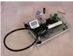
the scale at the bottom tops out at 400, no matter how much higher the actual reading shown on the numerical display. Readings are accurate to within 2 kg•cm<sup>2</sup>.
